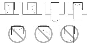
Print envelopes on the front address side only. Some parts of the envelope consist of three layers of paper-the front, back, and flap. Anything printed in these layered regions may be lost or faded.
