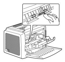
5 Align the imaging cartridge with the guides in the printer, and then insert the cartridge.
