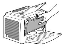
**3** Pull the handle of the imaging cartridge toward you, and then pull out the imaging cartridge.
