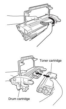
4 Using both hands, separate the toner cartridge and drum car-tridge.
