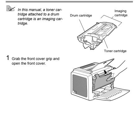
Replacing the Drum Cartridge
