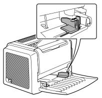
7 Load the envelopes lengthwise and the printing-side up as shown in the illustrations.
